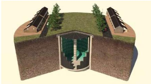
Figure 2: Ecovat vessel with constructive column in the center.
