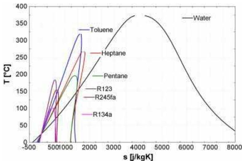
Figure 3. Saturation curve (Quoilin et al., 2013)
