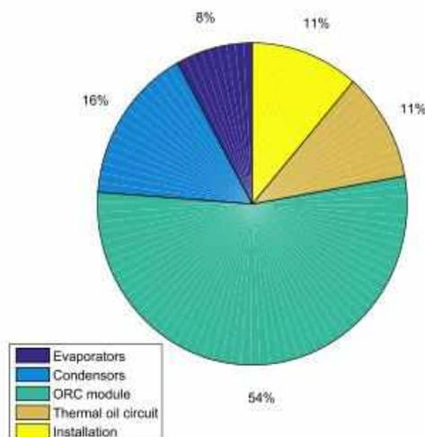
Figure 4. breakdown of the costs of an ORC system (Sanne Lemmens, 2016)
