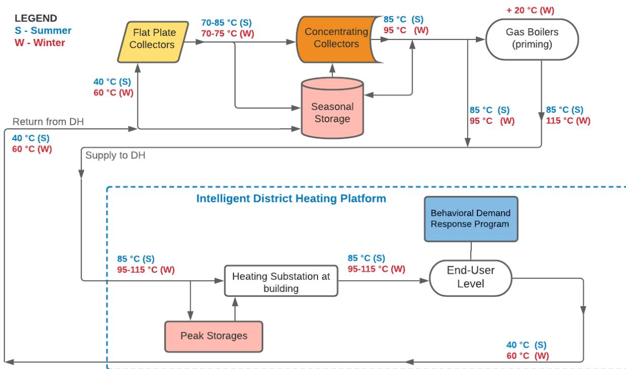
Figure 11- Complete Scheme of proposed solution including connections to DH network and temperature levels of supply/return for Summer and Winter operations
